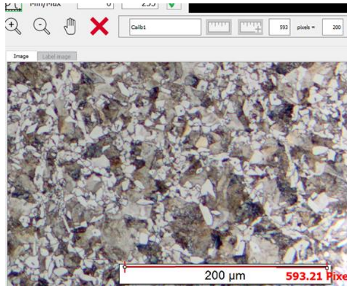
Figure 3: Positioning the calibration tool (in red) on the target displayed on the image.
